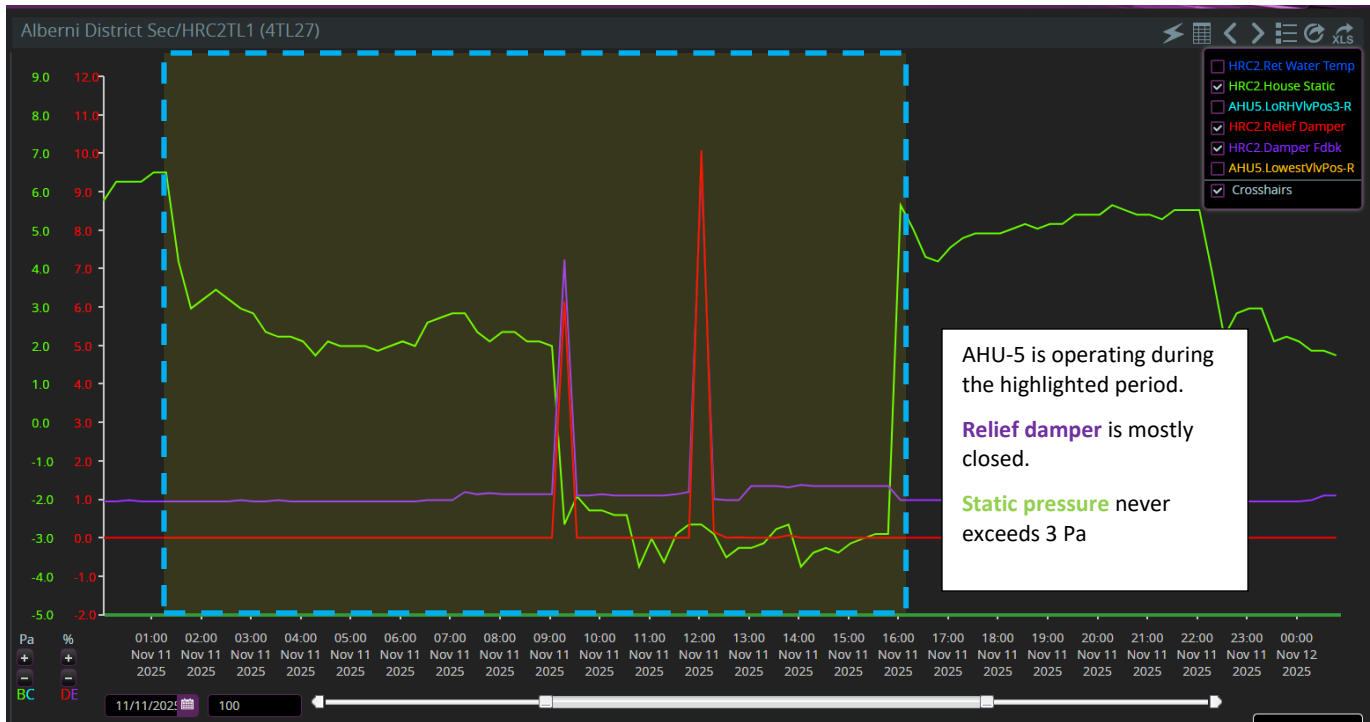
Figure 20: DDC Trend Log of the AHU-6 Relief Damper Position and the Measured Relief Hood Static Pressure
