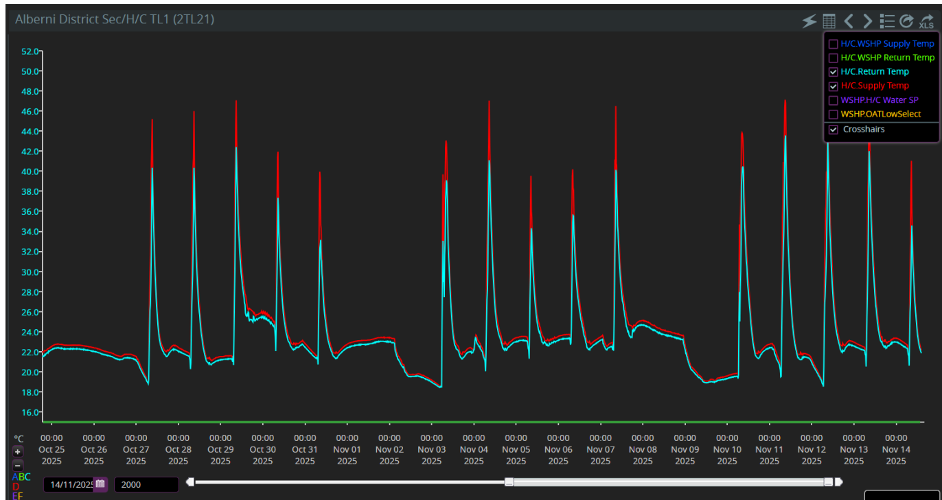
Figure 11: Trend Log of Hot Water Supply and Return Temperatures During a Period in October and November 2025
