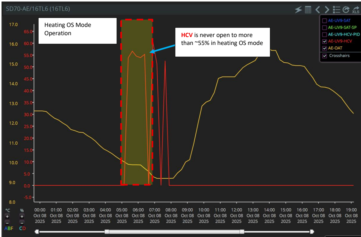
Figure 12: DDC Trend Log Data of UV-9 Heating Coil Valve (RED) and OAT (YELLOW)
