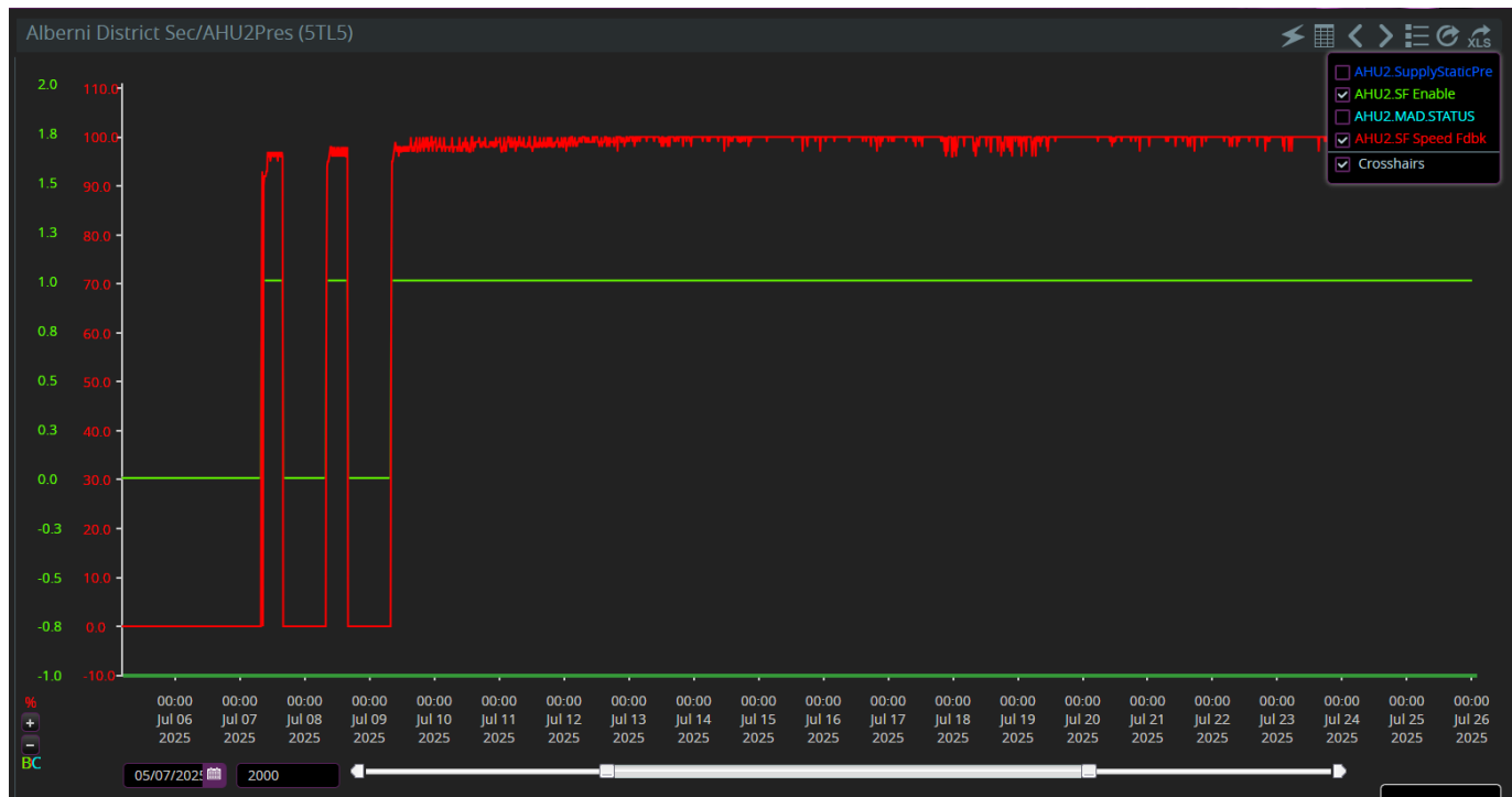
Figure 2: DDC Trend Log of AHU-2 Enable and Supply Fan VFD Speed in July 2025
