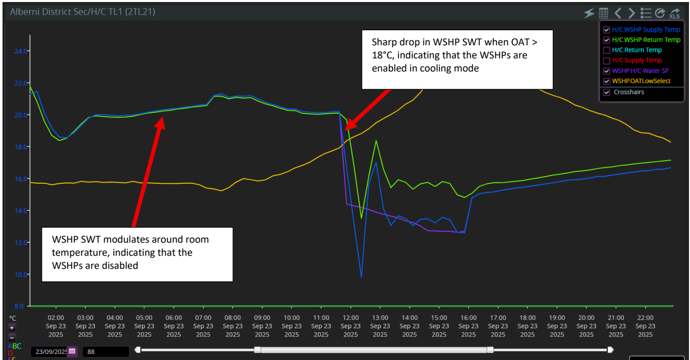
Figure 9: Trend Log of the WSHP Supply Water Temperature (BLUE), Return Water Temperature (GREEN), Supply Water Temperature Setpoint (PURPLE), and Outdoor Air Temperature (YELLOW) on September 23, 2025
