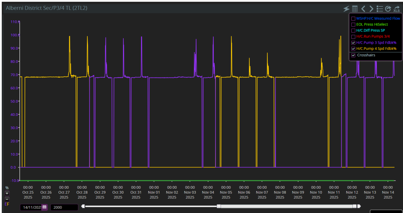
Figure 12: Trend Log of P-3 and P-4 VFD Speeds in October and November 2025
